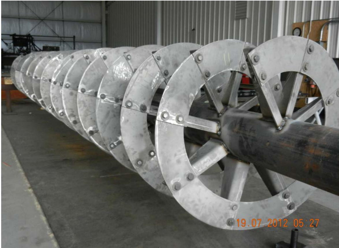
Above: Spiral Feed Transfer Auger Below Left: Elliptical GMax chamber
