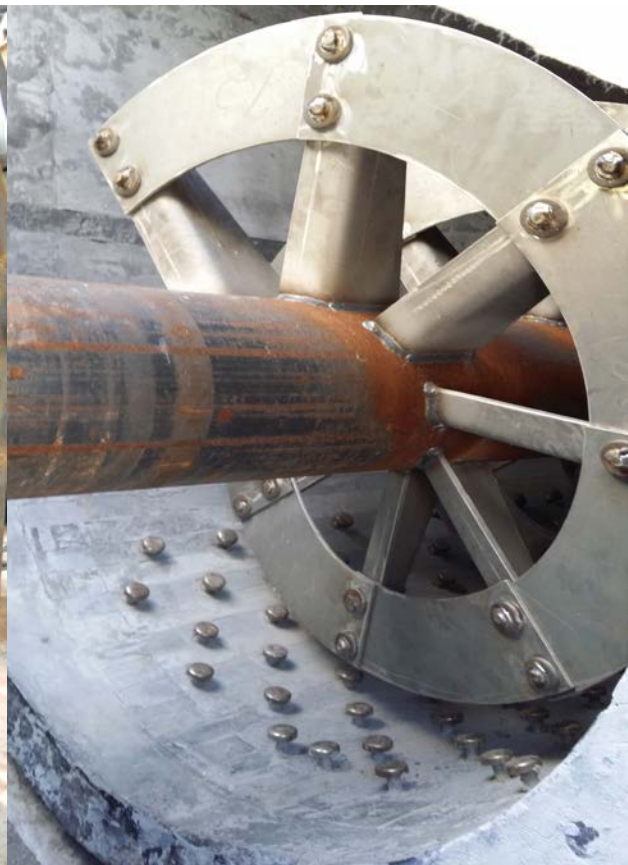
Below Right: Installed Auger, Bed Bubblers
