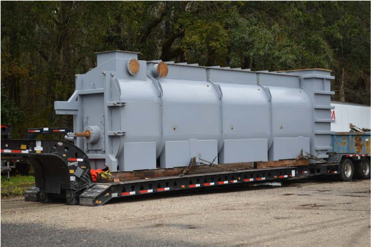
Fully assembled GMax Gasifier awaiting installation
